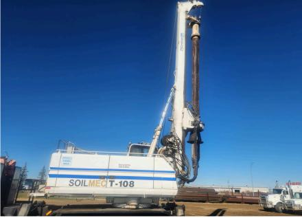
Mounted on a 2007 Peterbuilt 378 SBFA GVW 30,600 kg Max pile diameter 1800 mm Pile Max depth 30 m 14846 Hours SALE PRICE: \$265,000.00
