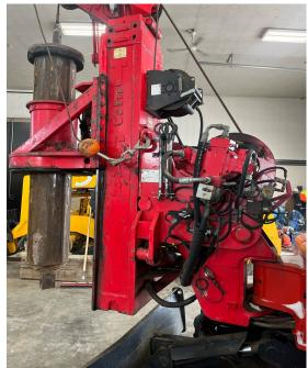
2135 Hours Small KB = 11 element, 30' depth Larger KB = 7 element, 68' depth 4 Augers Included -16" dirt, 16" rock, 24" dirt & 24" rock
