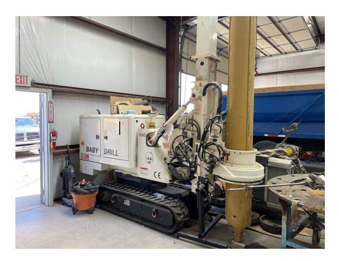
19 Hours - Stored indoors, torque - 12,900 lbsft 15 M interlocking Kelly Bar 11,900 lbs, Max Depth 59 ft, 8.2 ft Clearance
