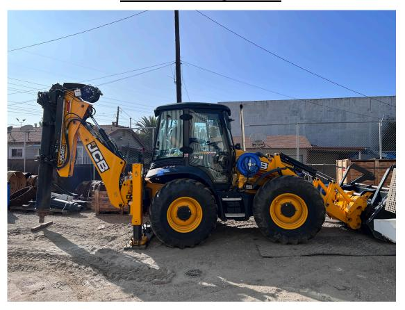
4CX Loader with built in Drilling Attachment
