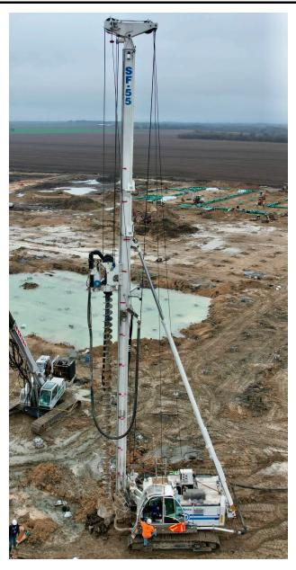
CFA Rig RATED TORQUE: 62,692 lb\*ft / 85 kNm MAX RATED DRILL DEPTH: 88.58 ft / 27 m
