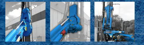
A range of rotary heads with different torques and drilling speeds to suit the various technologies. A new double rotary head setup to ensure high performance in a compact size and easy to be converted to single head.
