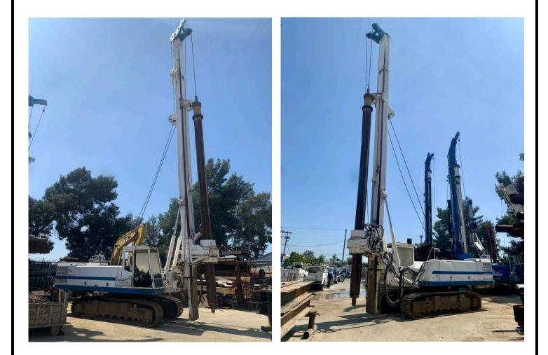
\*CURRENT HOURS: Meter in-op. Approx. 10,000 ENGINE TIER: T1 RATED TORQUE: 125,500 MAX RATED DRILL DEPTH: 130 ft. KELLY BAR: 5x25.5'
