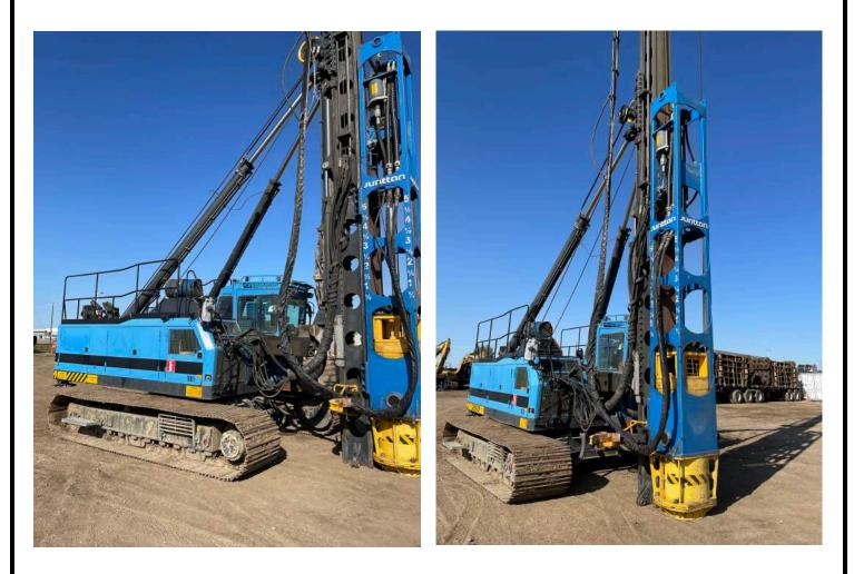
HHK 4SL Hydraulic Impact Hammer: Max Energy: 43,517 ft-lbs Drop Height: 2 – 59.1 Inches Blows per Minute: 30 – 100 Ram Weight: 8,818 Pounds Total Weight: 15,873 Pounds
